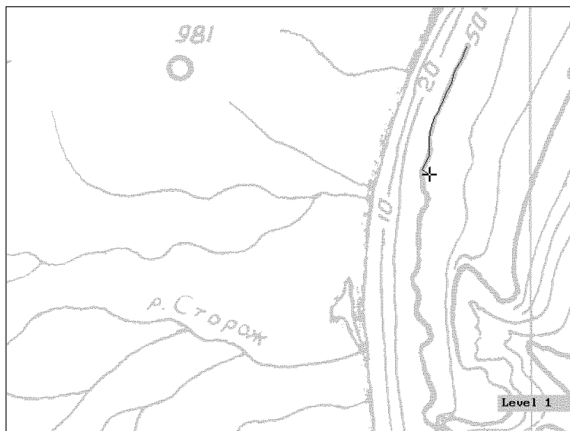
Figure 4. Process of digitizing in manual mode. User moves cursor along lines and inputs its coordinates by clicking mouse button. Inputted segment is drawn with black color
