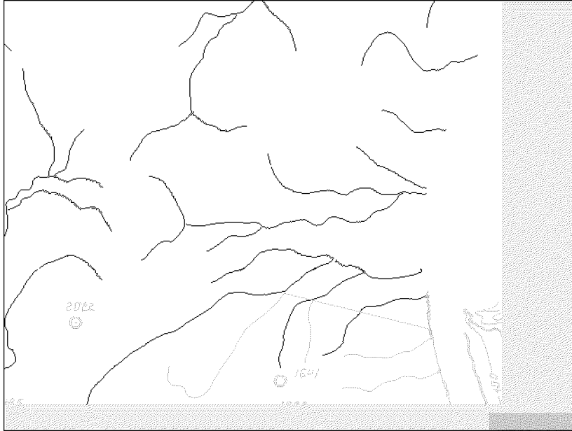
Figure 6. The procedure of the vector data cleaning. Saved data is drawn with black color. All the vector data after automatic vectorization is drawn as gray lines
