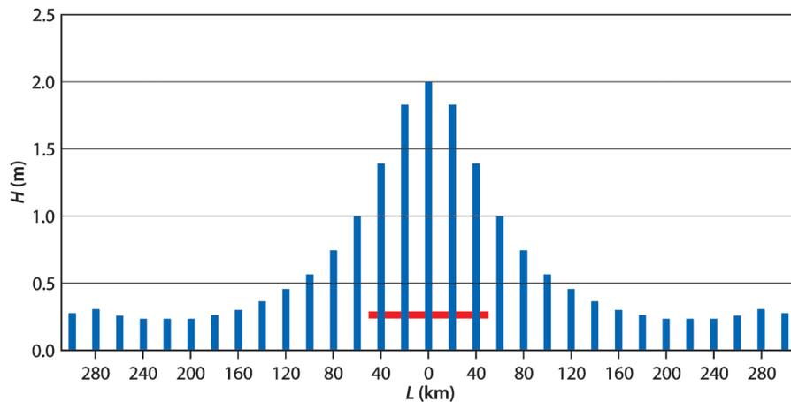
**Fig. 14.4.** Typical distribution of tsunami run-up heights along the coast calculated for a model source equivalent to a magnitude 7.5 submarine earthquake. Section of the *solid line* shows the position and size of the seismic source
